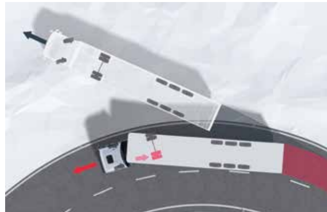
ESP compensatory braking when vehicle is understeered.
