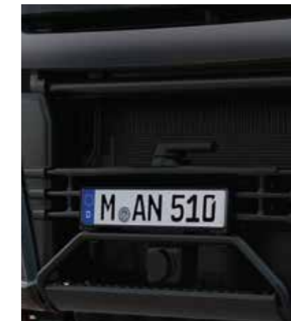
Steel bumper with centred towing eye and hinged front step. Particularly robust protective grille in front of radiator.
