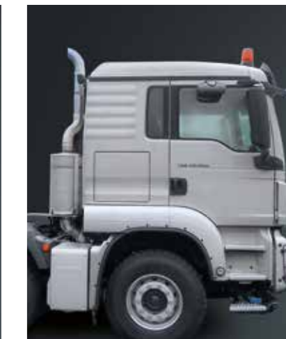
Partially raised exhaust system for L cab
