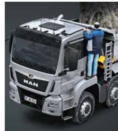
Construction-site rise with support rail on roof.
