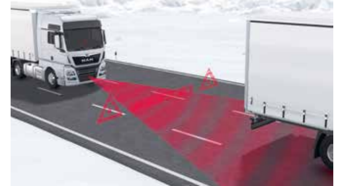
Functional principle EBA: advanced traffic monitoring by using two independent sensor systems (radar and video)
