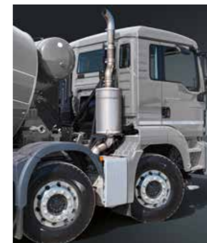
Partially raised exhaust system
