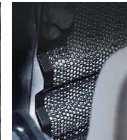
Protective guard in front of radiator
