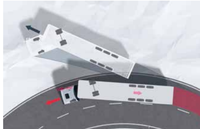
ESP compensatory braking when vehicle is oversteered.
