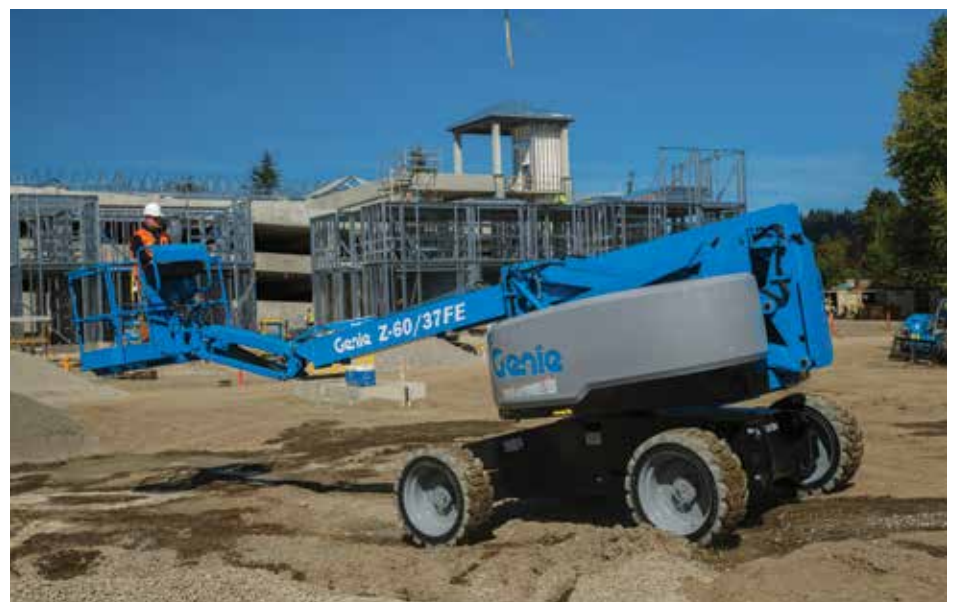
A true 4-wheel drive articulating boom with fully sealed AC drive motors
